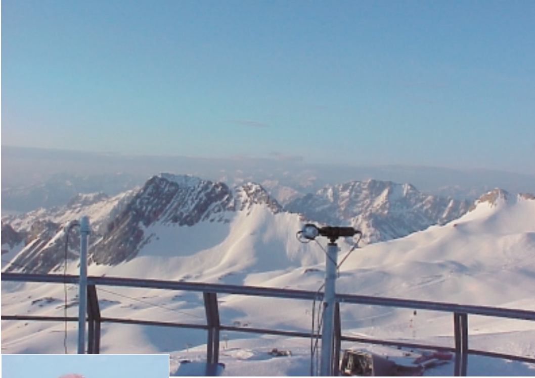
The ASCARATIS system measures UV radiation, weighted according to its capacity to produce sunburn – here in the skiing region of Mount Zugspitze.
