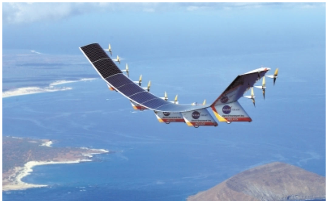
Solar cells and an ultra-light aerofoil construction using composite fibre materials allow the Helios solar aeroplane to fly at a height of 23 km. (Photo: NASA)
