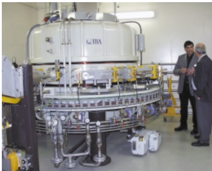
The electron accelerator at Saal an der Donau provides more than 10 MeV acceleration energy, and a beam power of 150 MW.
