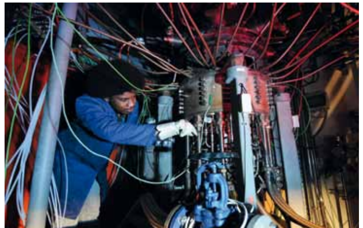
Test facility of annular combustion chamber (Source: Chair of Thermodynamics, Technical University of Munich)
