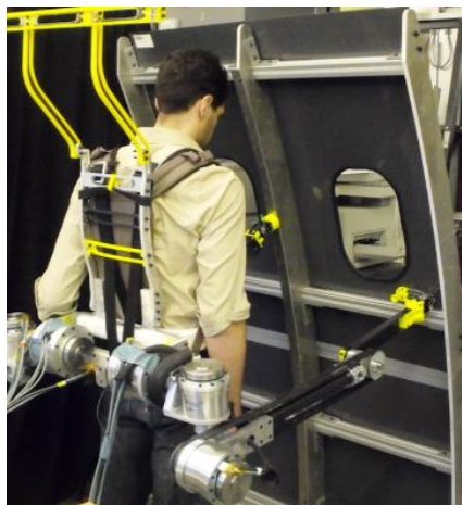
SRL variant 1: prototype used in a drilling task (Image: © [2014] IEEE. Reprinted, with permission, from Parietti and Asada, 2014)
