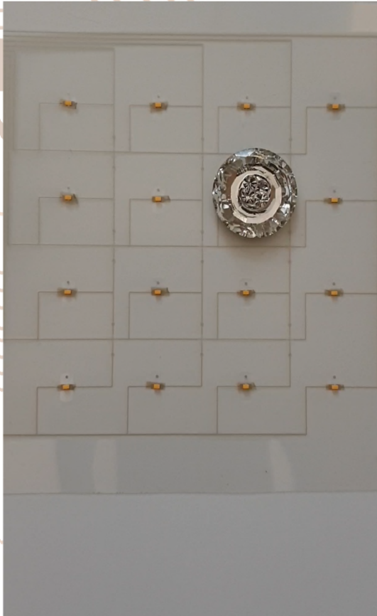
1st version crystal LED array
