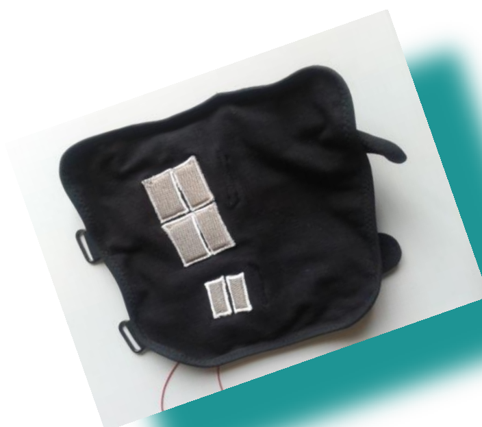
Prototype panel containing 6 textile electrodes.
