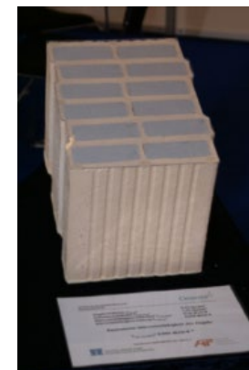
CALOSTAT- brick \lambda_{\text{equiv.}} = 0,041 \text{ W/(mK)}
