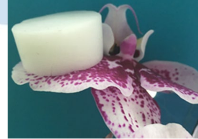
Modified silica aerogel
