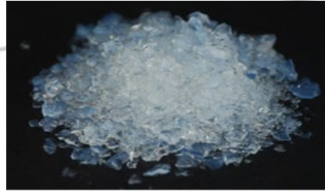
SiO 2 - Aerogel \lambda_{10, \text{tr.}} = 0,023 \text{ W/(m} \cdot \text{K)}
