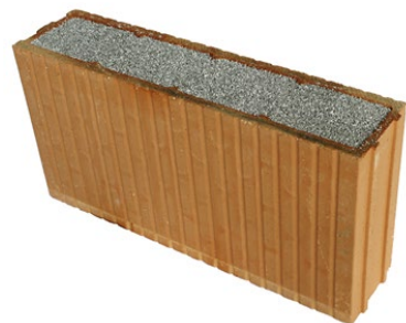
Perlite-brick \lambda_{\text{equiv.}} = 0,071 \text{ W/(mK)}
