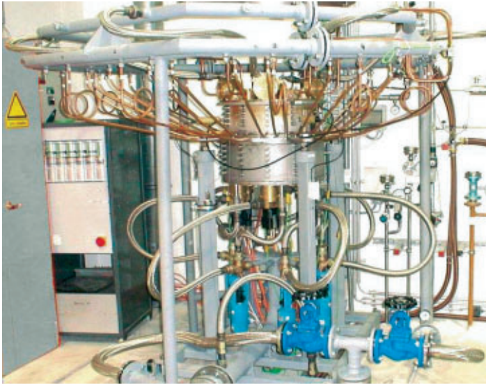
Annular combustor test rig of a gas turbine for thermo-acoustic measurements.
